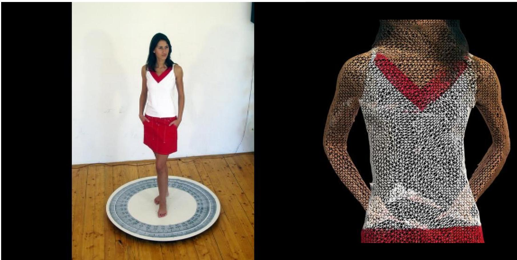
Fig. 17. Scanning with digital Body Capture System "BodySABA 0.3." and digital 3D presentation of the object scanned in Wireframe
