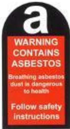
Figure 6: Marking for asbestos-containing waste
